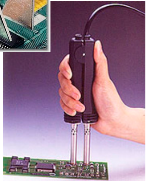
Right: SMD rework by conduction heating uses heated "tweezers" to heat all of the pins at once.
