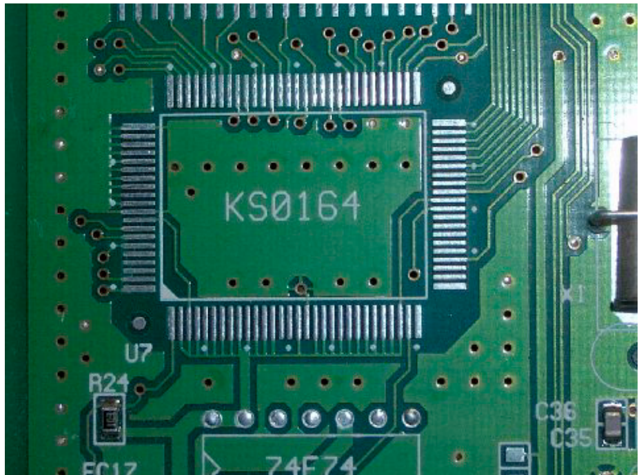
Clean pads - Ready for the new device to be installed!
